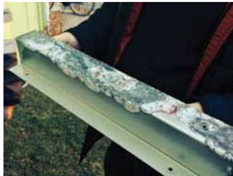
Figure 6: The zink covering of the steel profile is corroded as a result of direct contact with salty sweat or 'tear' drops from the adjacent MgO-board.
